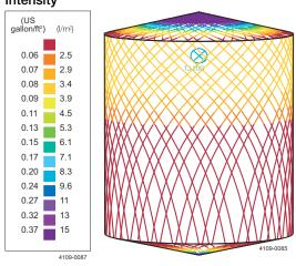
D4.6 m H5.5m, Toftejorg MultiJet 25. 4  $\times$  5.5 mm, Time = 2.08 min, Water consumption = 403 I
