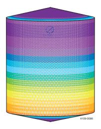
D4.6m H5.5 m, Toftejorg MultiJet 25. 4 x  $\varnothing$ 5.5 mm, Time = 8.3 min, Water consumption = 1612 I
