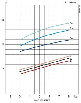
A: Wetting B: Impact cleaning  $A_1 = 4 \times \emptyset 5.5$   $B_1 = 4 \times \emptyset 5.5$  $A_2 = 4 \times \emptyset 4.6$   $B_2 = 4 \times \emptyset 4.6$  $A_3 = 4 \times \emptyset 3.9$   $B_3 = 4 \times \emptyset 3.9$
