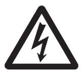
Electrical equipment An electric shock can injure or kill. Treat all electrical equipment as powered. Switch off power before maintenance or repair.
