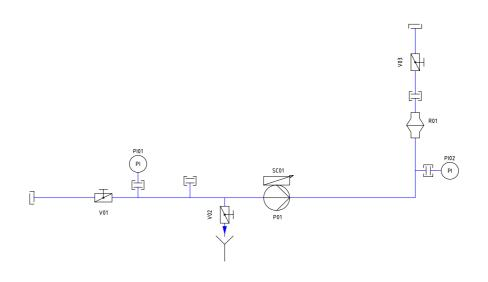
On the suction side of the pump there is a manual butterfly valve, a pressure gauge and a blind connection plus a drain.
