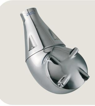
the tank. The nozzles rotate around both the horizontal and vertical axes in a 360° movement. This three-dimensional jet rotation enables the jets to reach the entire tank volume, providing fast, efficient mixing of the injected liquid, gas or powder without requiring batch rotation.
