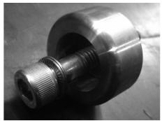
Figure 12, Bushing for shaft / gear motor
