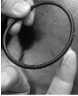
Figure 6, Greasing O-ring
