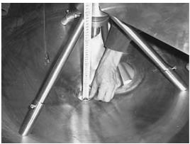
Figure 2, Height of Bottom Console
