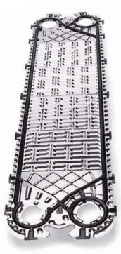
WideStream: Our WideStream plates with clip-on gaskets have very few contact points, which helps prevent blockage and results in longer uninterrupted operating times. Available only for Alfa Laval FrontLine, the plates are specially developed for the pasteurization of fruit juices and other products containing a limited amount of pulp and fibres.
