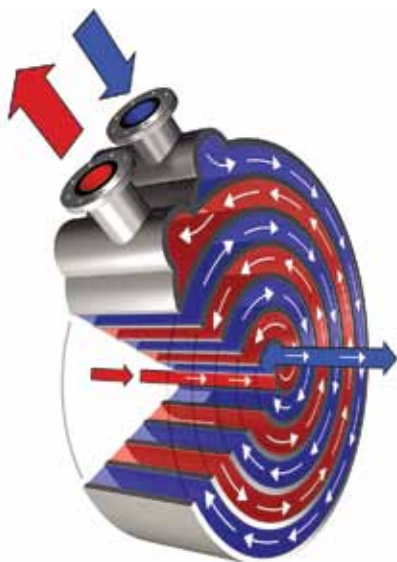
FIG. 2 Single-channel geometry resists plugging while counter current flow efficiently recovers heat.
